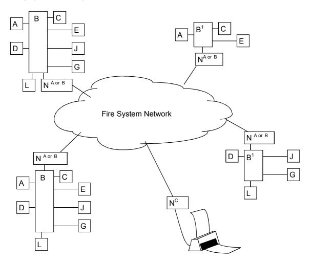
Figure B1: Example of a Fire System Network in relation to Control and Indicating Equipment
