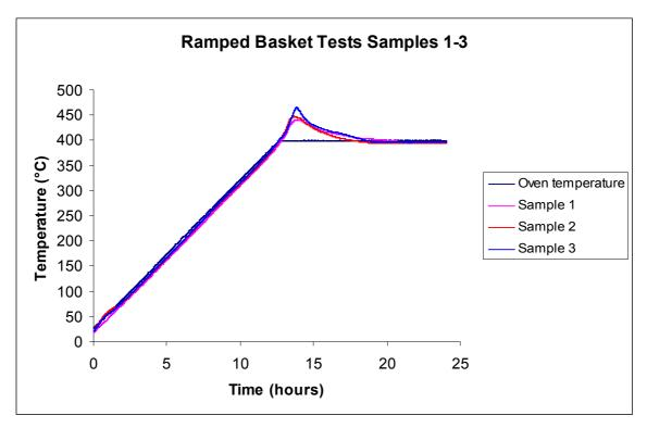
The figure above shows a test trace for a material exhibiting self-heating behaviour.
